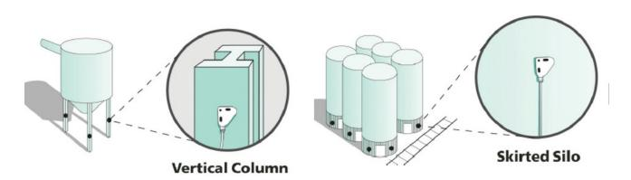
AccuBin Sensors are Bolt-On Strain Gauges that attach to a Silo's Steel Skirt or Legs. These Sensors along with Special Cloud Based Algorithms achieve Inventory Accuracies of 2-5% of the Weight of Silos Contents. Wireless Communications eliminate the need to Hard Wire the Data back to a Host Computer.
